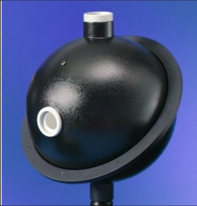
The model 2500 is a six-inch diameter integrating sphere with a 3/4 inch entrance port. It is suitable for both laser power measurement and LED photometry. It is compatible with Standard Series sensors.
